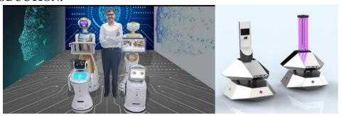
Invento C-Astra, a robot which helps screen patients and to disinfect common areas. The autonomous mobile unit can move around lobbies, hallways and can sanitise rooms. According to the startup, the robot makes use of disinfecting UV-C lamps to disinfect a room completely in just three to four minutes. The robot is currently being used in hotels to disinfect rooms, and is also being used at Apollo Hospitals, etc.
